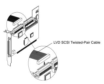
Figure 1-5. LVD SCSI Twisted-Pair Cable
